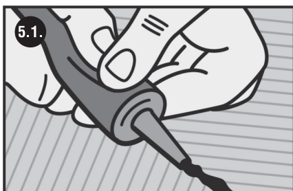
5.1. Detailansicht Nahtversiegelung Detailed view of seam sealing
